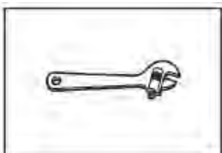
10" (254 mm) adjustable wrench that opens to 1 1/8" (29 mm)
