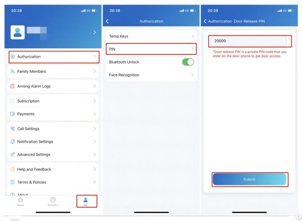
After you set a PIN code, you just need to enter the code on the keypad (depending on the door units model, the keypad could be a softpad or a physical one) to make the door open.
